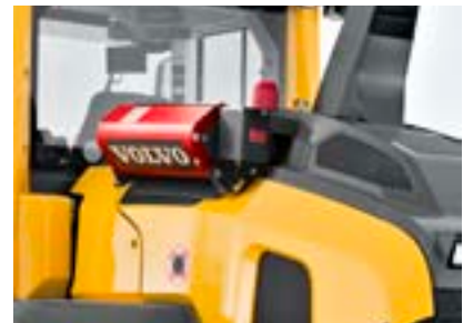
Fire suppression system
